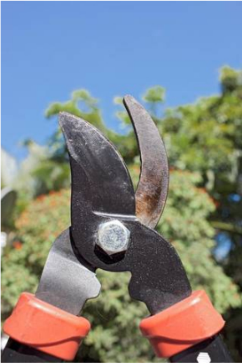
Lopper blades dry and oiled. The bolt allows for tightening. Kenneth Setzer - Fairchild Tropical Botanic Garden
